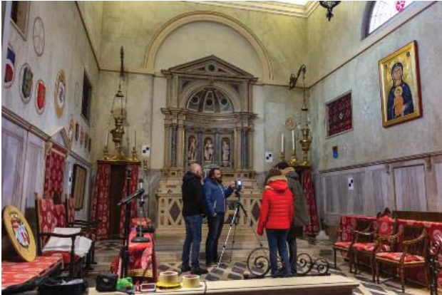
Figure 2. Laser scanning survey of the High Altar in the Church of San Giovanni Battista in Venice
