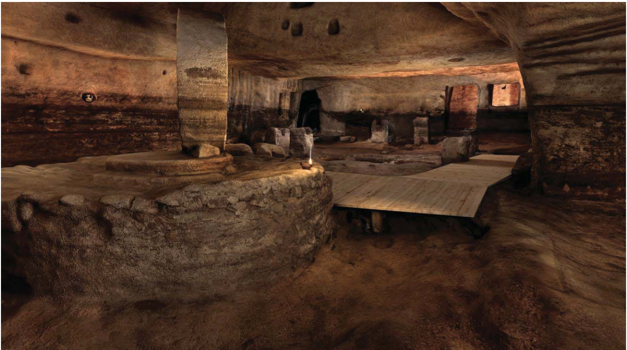
Fig. 3: 3D model based on digital photogrammetry. Here two sets of images were used, the first to obtain the 3D model and the second to ensure optimal texturing.
