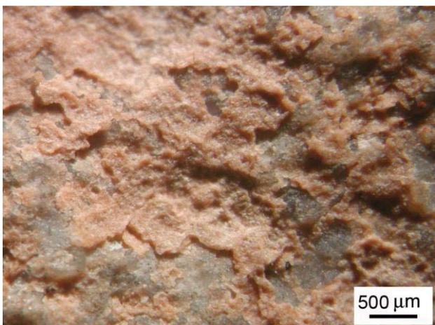
Fig. 7. Aspect of Ca-oxalate film (type 1) in St. Geminiano Church under stereomicroscopic observation
