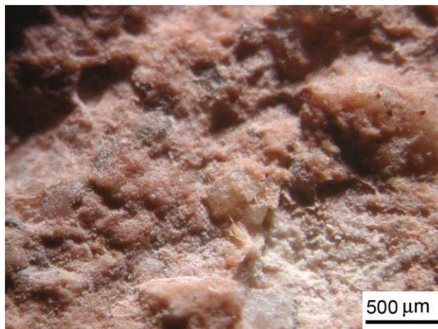
Fig. 5. Aspect of Ca-oxalate film (type 1) in St. Antioco di Bisarcio Basilica under stereomicroscopic observation
