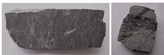
Fig. 4. Photographs of selected samples (the thickness of the samples is about 10 cm): on the left, a RET sample with white thin intersecting veins of calcite; on the right, a SVL sample characterized by typical chromatic alteration (from black to gray) and by the presence of a centimetric black flint.
