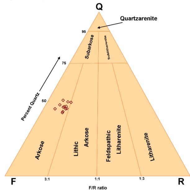
Fig. 1: QFR diagram for Folk's sandstone classification. The analysed samples can be classified as arkose/lithic arkose.
