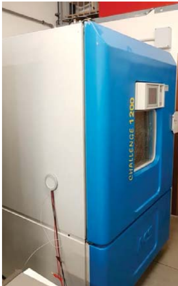
Fig.4. Challenge 1200 ACS oven chamber.
