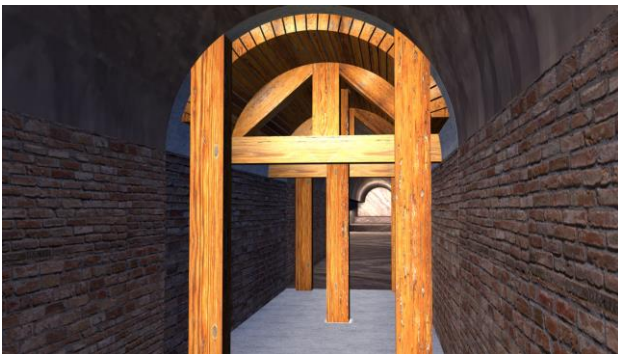
Fig. 5. Virtual reproduction of the centering used in the Roman works. It is based on the structures found by Torlonia's engineerings, as described in their publications.
