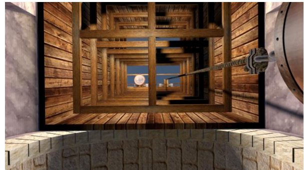
Fig. 6. Reproduction of the Roman wells scaffolding, found intact during the nineteenth century works.
