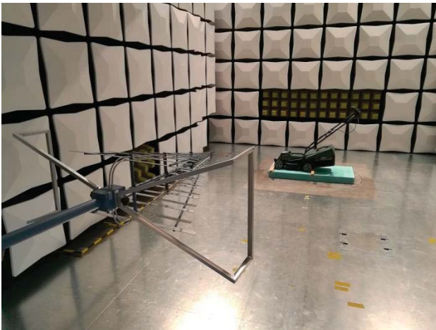
Fig. 1. Measurement setup of radiated emission measurement
