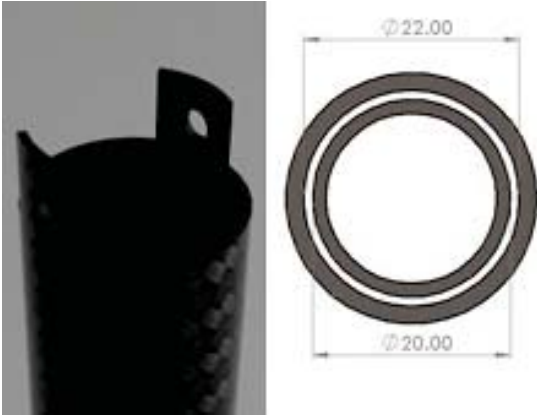
Fig. 4. Carbon fiber sensor rendering (left) and dimensions (right)
