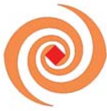
Fig. 2. Computer model of planar log spiral antenna to 0.9 GHz.
