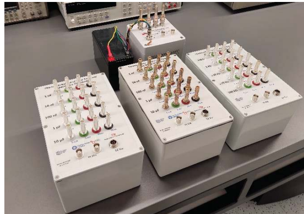
Fig. 1. 4TP resistance and capacitance standards used at GUM and SUT (two sets of thermostated capacitors and one set of thermostated Vishay resistors – at the bottom from the left, and 10 nF thermostated capacitors with battery – at the top).
