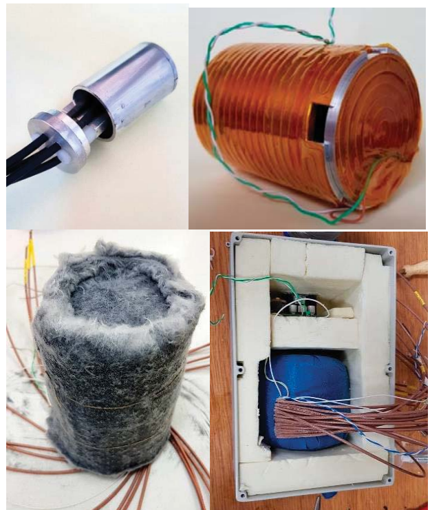
Fig. 2. Stages of construction of the thermostated set of standard capacitors (shielded housing with a single capacitor – top left, enclosure with heating foil – top right, set of five capacitors mounted in the heating enclosure and insulated with aerogel – bottom left, complete set without cover – bottom right)
