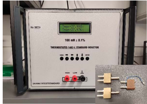
Fig. 4. Thermostated standard inductor 1482-L. Modified by Ukrainian NMI. The MUSA adapter and the MUSA tees are visible in the small window at the bottom right
