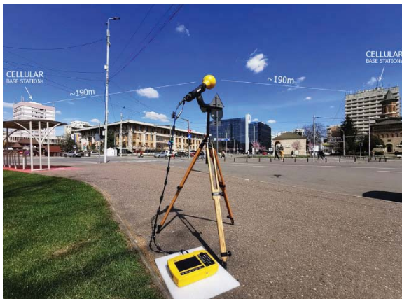
Fig.2 Narda SRM 3006 field strength analyzer
