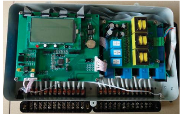
Fig. 2. Internal structure of multi-user electric energy meter.
