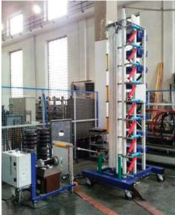
Fig. 2. LATFC's Haefely Impulse generator.
