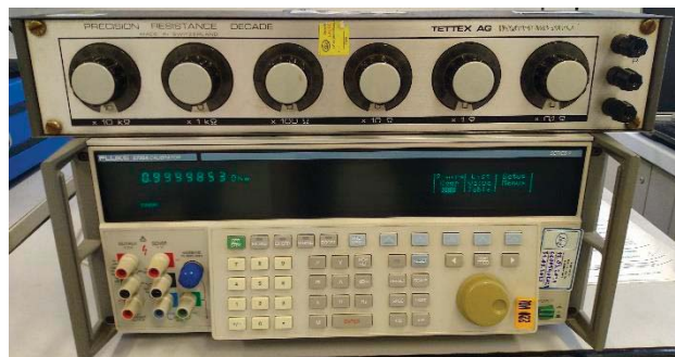
Fig. 2. Tettex 1108-B GR decade box and Fluke 5720A MFC working standards.
