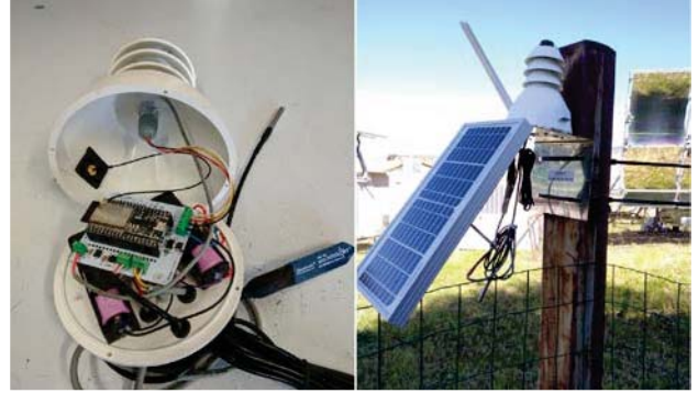
Fig. 2. Images of the developed sensor node. On the left side a detail of the boards enclosed inside a waterproof case, while the right image shows the whole node installed on the field (including the photovoltaic panel).
