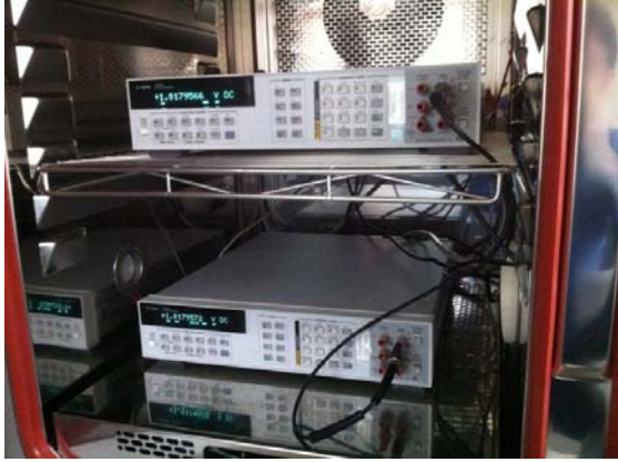
Fig.3. View of the set-up for the evaluation of temperature influence on the frequency response of two DMM in the DCV sampling model.
