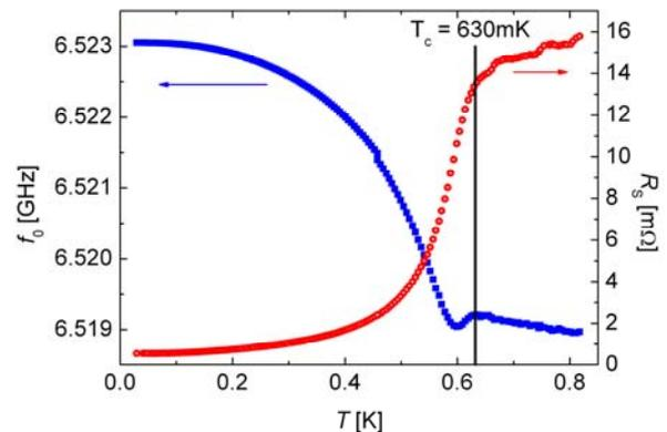
Fig. 3. Temperature dependence of stripline resonator frequency  $f_0$  and sample surface resistance  $R_s$  measured on a CeCu<sub>2</sub>Si<sub>2</sub> single crystal sample.
