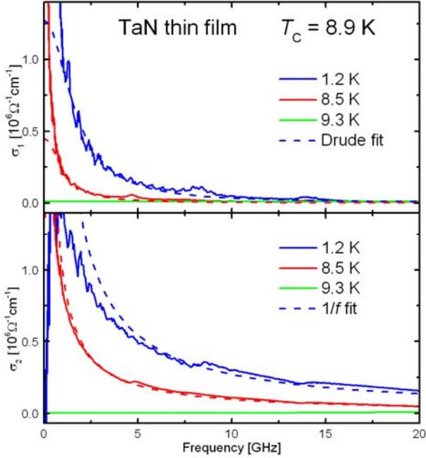
Fig. 2. Microwave conductivity spectra of a TaN thin film, measured with a Corbino spectrometer.
