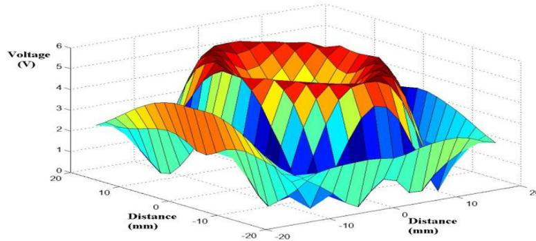
Figure 2: A graph of voltages seen in the field of the NFC enabled device.
