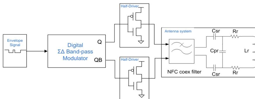
Figure 3: Block diagram of proposed single-bit transmitter architecture
