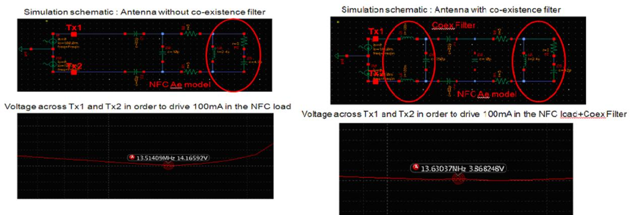
Figure 11: Simulation of the NFC antenna with and without the co-existence filter
