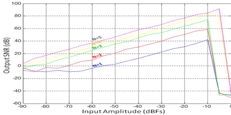
Figure 8: SNR versus Input Amplitude Sweeps for different number of bits in the quantizer
