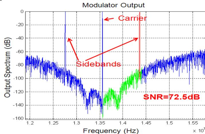
Figure 9: 4-bit modulator output spectrum with 100% ASK signal
