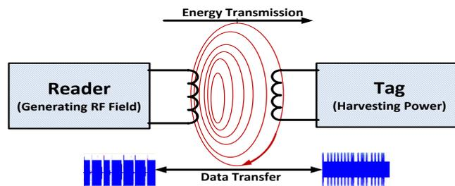
Figure 1: Block diagram illustrating a basic NFC system
