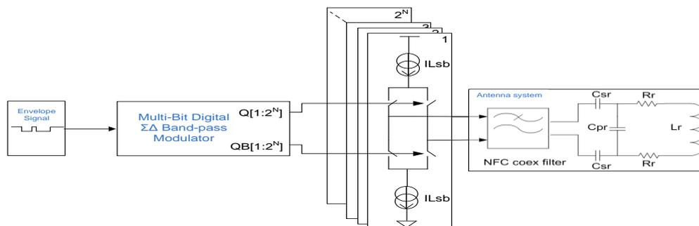
Figure 7: Block diagram of proposed multi-bit transmitter architecture
