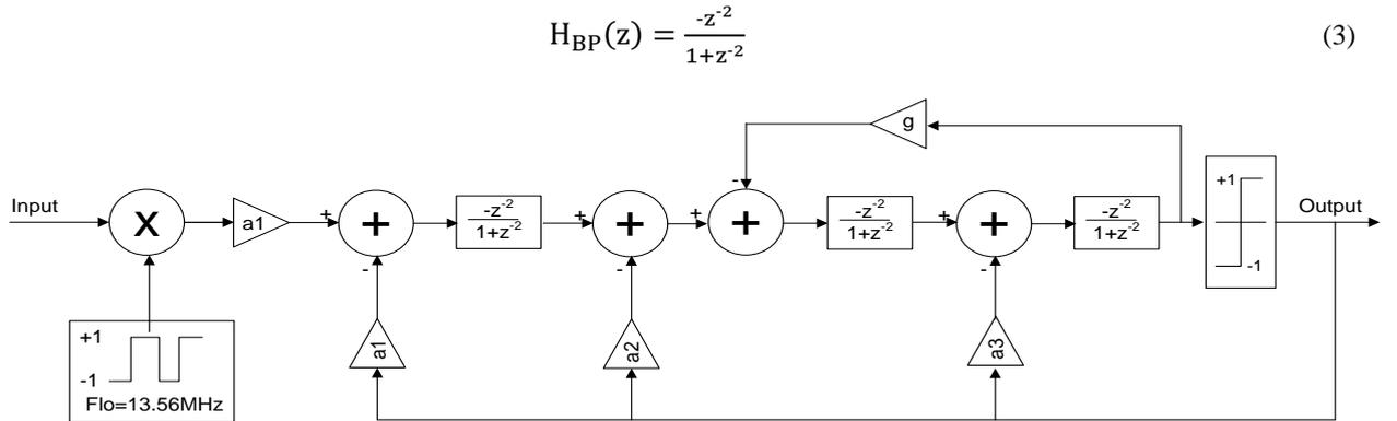
Figure 4: Block diagram of the band-pass modulator
