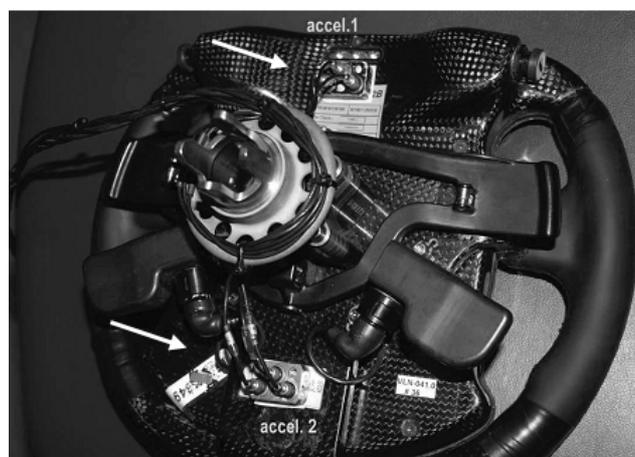
Fig. 4. Accelerometers positioning on steering wheel.
