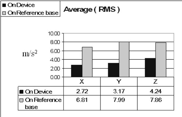
Fig. 5. Time domain vibration on steering wheel base and electronics.
