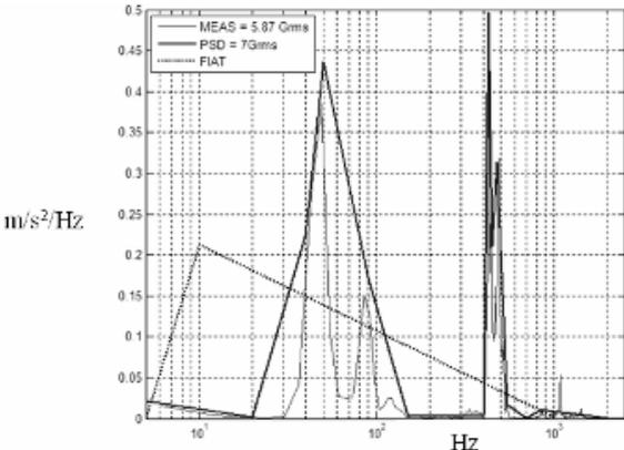
Fig. 7. PSD vibration test on kerbs.
