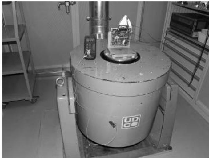
Fig. 1 Shaker system Unholtz-Dickie, model TA115SA-40.
