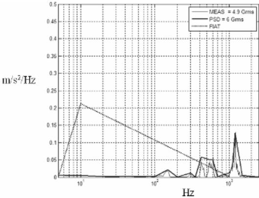
Fig. 6. PSD vibration test on straight line running.
