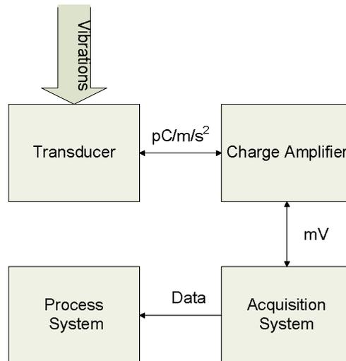
Fig. 3. Block scheme of vibration measurement system
