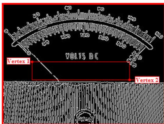
Fig. 4. Binary image of the display obtained after the Canny's method and its corresponding region of interest (ROI) selected by the user.
