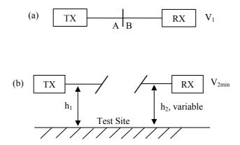
Figure 1. Schematic showing arrangements for measuring  $V_1$  (a) and  $V_{2min}$  (b). In (b) RX is height scanned.
