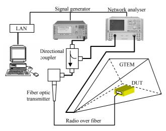
Figure 6. Experimental setup for measurements on a DUT inside a GTEM test cell.
