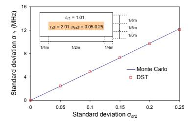
Figure 7. Standard deviation of the resonant frequency as a function of the standard deviation of the slab dielectric constant calculated with Monte Carlo and DST techniques.
