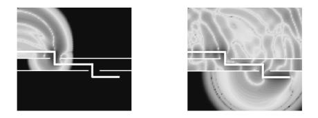
Figure 4. Magnetic field associatted with a pulse propagating through a cascade of vias.
