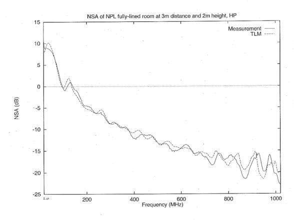
Figure 3. NSA in fully tiled room (horizontal polarization).
