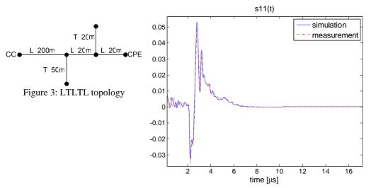
Figure 4. The comparison measurement-simulation for L(LTL)L topology
