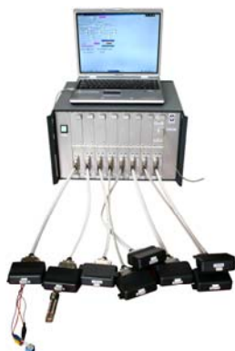
Figure 4. Multi-channel electrochemical supercapacitor measurement system
