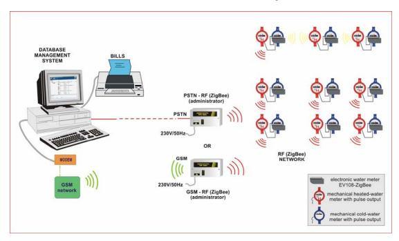
Fig.1. Wireless automatic water-meter reading system
