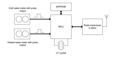
Fig.2. Schematic diagram of WMU
