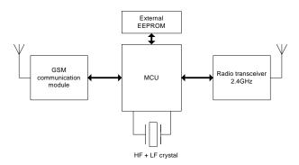
Fig.3. Schematic of data collector
