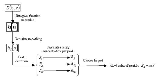
Figure 3: Flowchart of the ambient illumination conditioning algorithm applied to each colour channel of the image difference
