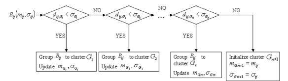
Fig 4. Flowchart of the image block clustering algorithm
