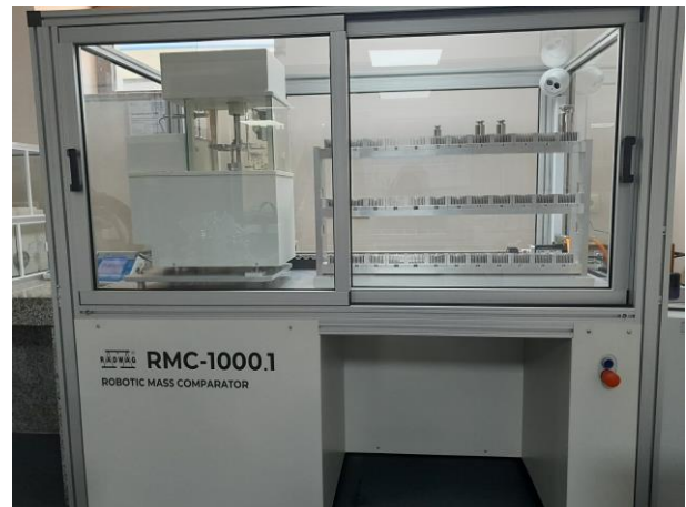
Figure 3: The new RMC 1000.1.5Y comparator during repeatability tests
