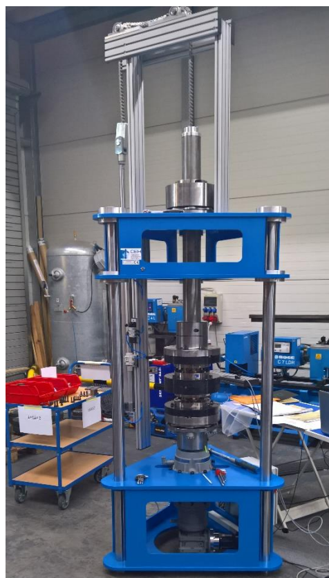
Figure 1: The 20 kN·m TCM at NMISA
