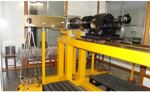
Figure 2: The 3 kN·m TSM at INMETRO
