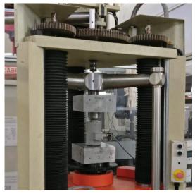
Figure 1: The 20 kN transducer placed between the  $3^{\circ}$  tilted plates integrated into the MCF30 FSM
