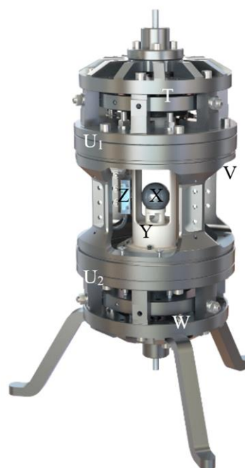
Figure 1: NPL Demonstration Kibble Balance showing the support frame (V), moving frame (Y), spherical mass (X), encoder read-head (Z), tare magnet and coil (T), weighing magnet and coil (W), and two disk flexures (U 1 and U 2 )
