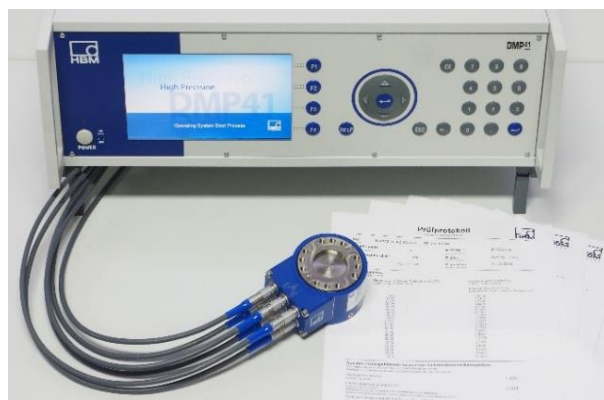
Figure 2: DMP41 can e.g., be used to read out the 6 forces & moments measured by MCS10 multi-axis transducer
