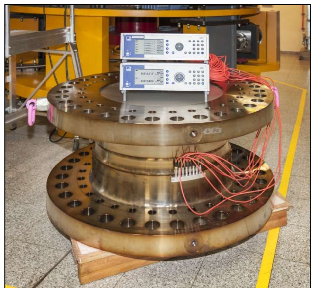
Fig. 2. 5 MN·m torque transducer together with two DMP41 bridge amplifiers for the readout of the eight channels of the transducer.
