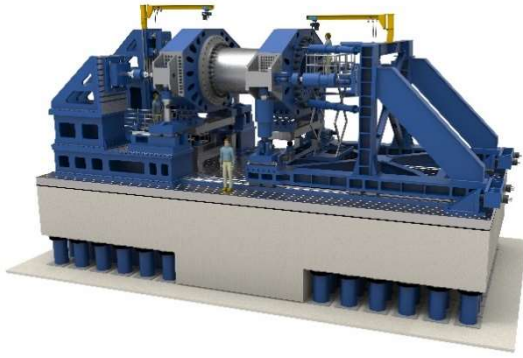
Fig. 6. Design of a new standard torque calibration machine for torques of up to 20 MN·m.
