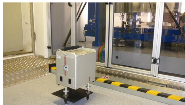
Figure 2: Lower part of the 200 kN FSM with gravimeter Scintrex CG3M-4492.
