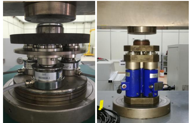
Fig. 4 BU 2 and BU 4 were tested in the 300 kN DWFSM
