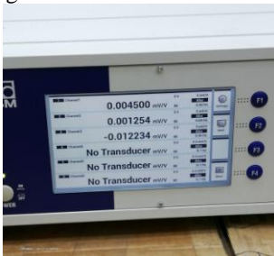
Fig. 7 Data were indicated by DMP 41 and taken by a software every 0.2 s
