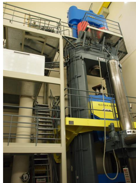
Fig. 2: PTB's 16.5 MN force standard machine
