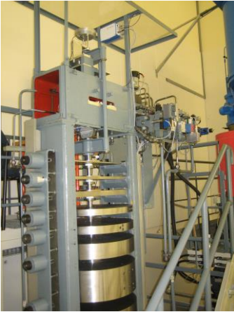
Fig. 3: Deadweight side of the 16.5 MN fsm
