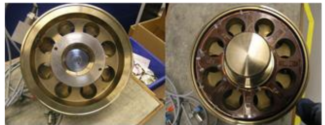
Figure 2.3: Force transducer Top – Z4a/500KN. Completely monolithic structure of the spring body.
