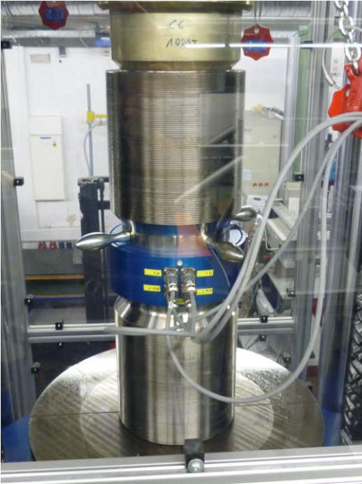
Figure 4.1: 6.5MN Tension bar in the 5MN calibration machine of HBM.
