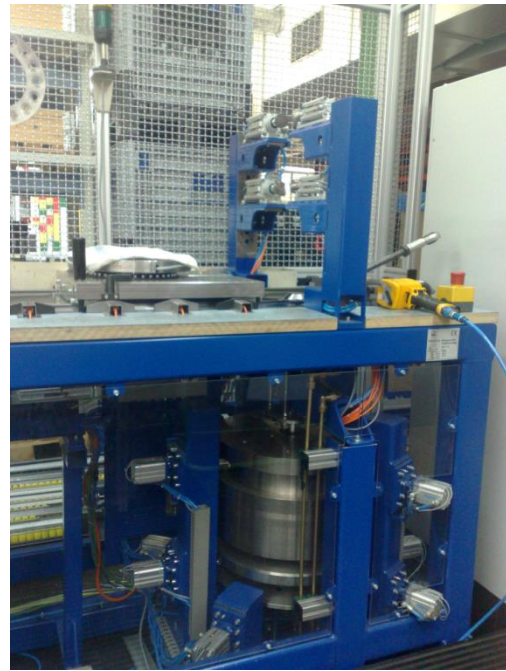
Figure 3.2: Machine for the introduction of bending moments. The sensor is mounted on the plate (left) the weights (right, button) are applied over a lever arm. The sensor turns while measurement so that a constant bending can be applied all directions.
