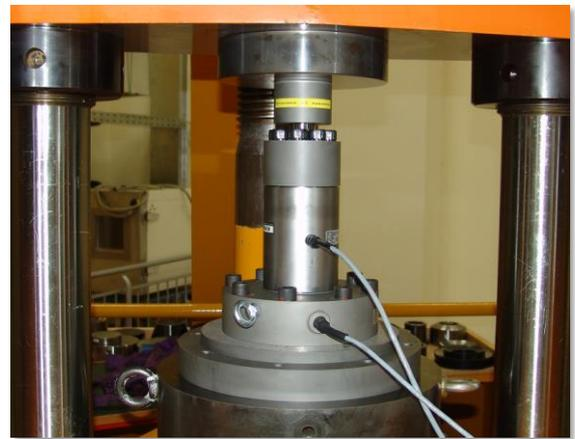
Fig. 5: The figure shows the build-up system mounted in the 1MN force standard machine (fsm) of PTB.
