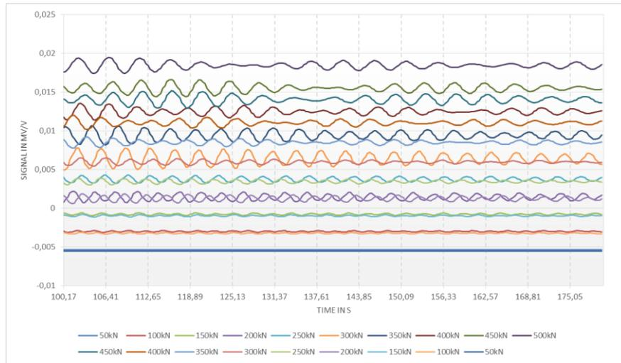
Fig. 6: The diagram shows the oscillation of the fsm masses. It caused an additional torque into the CT-transducer system. You can see the correlation for a up-down cyclus of 10% load steps.
