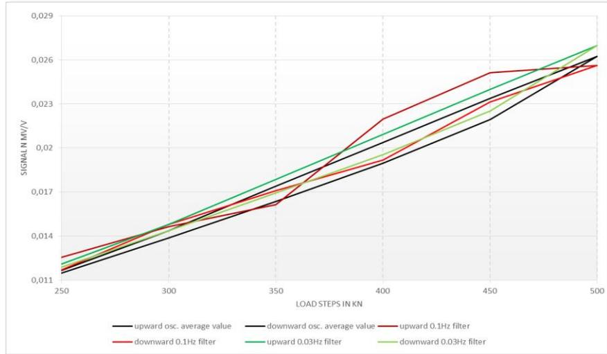
Fig. 9: The diagram shows the comparison of the calculated average values and the values calculated by the amplifier using different low pass filters. It shows that only the using of a low pass filter with 0.03 Hz makes sense.
