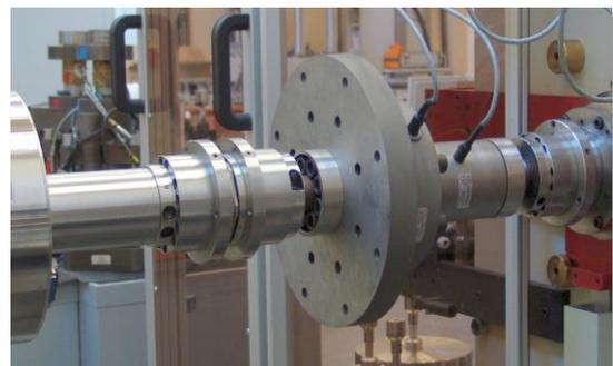
Fig. 2: The figure shows the build-up system mounted in the 1kN·m torque standard machine of PTB.
