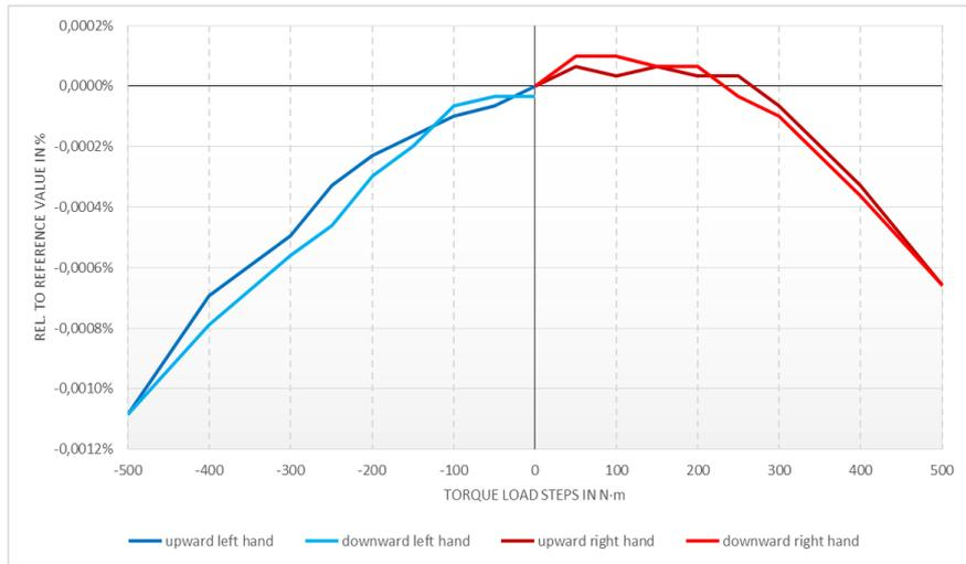
Fig. 3: The diagram shows the influence of a torque applied on the force transducer. The force transducer has a dependence to the applied torque step but the small relative crosstalk influence is still negligible.
