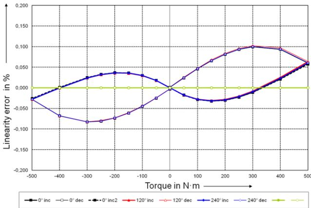
Fig. 4: The diagram shows the linearity error of the sensor during the calibration at a torque of up to 500 N·m which is oriented towards the left and towards the right.
