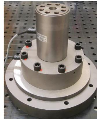
Fig. 1: The figure shows the build-up system consisting of a force transducer and a torque transducer which has been investigated with regard to its crosstalk behaviour.
