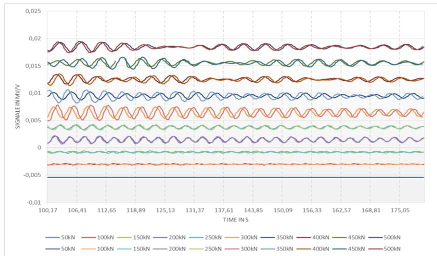
Fig. 7: The diagram shows the comparison of two measured oscillation at the same CT-transducer position. It shows a high repeatability of the oscillation characteristics like amplitude and phase.
