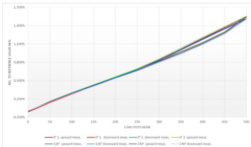
Fig. 8: The diagram shows the calculated average values of the oscillation over a measuring time of 300 s. There is a dependence of the transducer position but the functional relationship is nearly identical.
