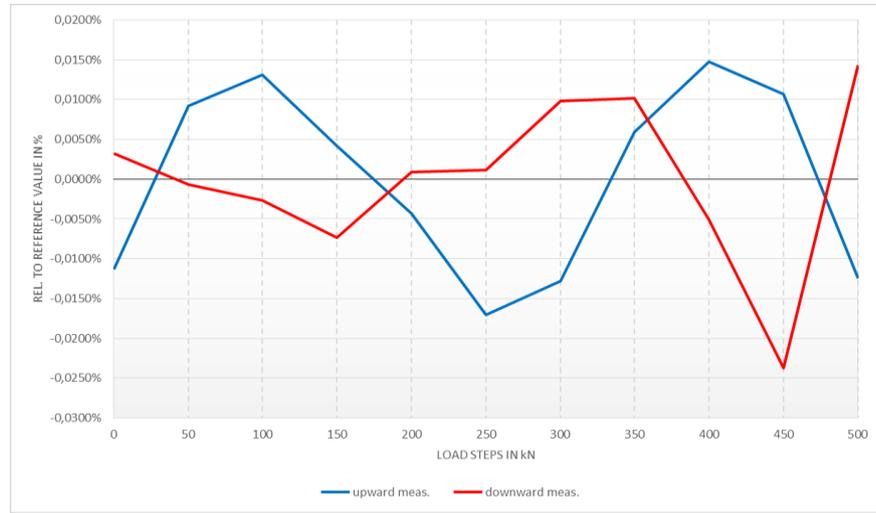
Fig. 10: The diagram shows the remaining influence of an applied force to the torque transducer by using the fit functions of Tab. 1.
