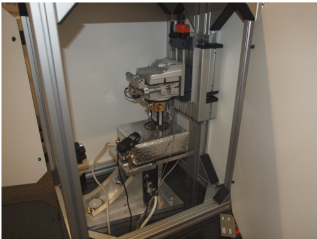
Fig. 3. Photograph of the new FSM. In the lower part one can see the NPT and the balance, surrounded by a foil to reduce thermal influences. Above the balance, the transducer, with the adapter mounted on the rotational and tilt table.
