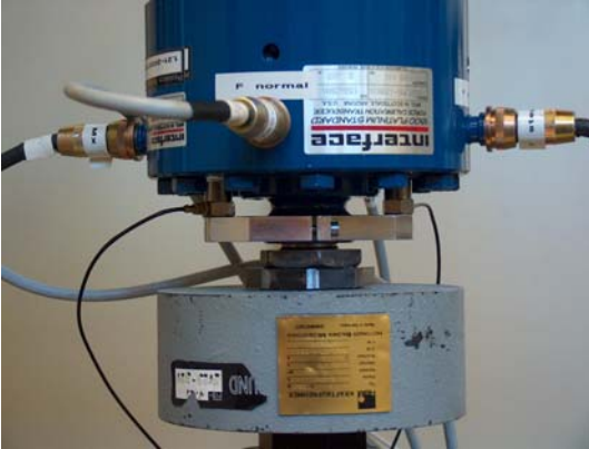
Fig. 6. Arrangement of the two force transducers and the acceleration transducers
