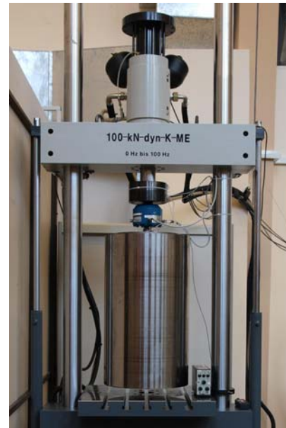
Fig. 3. Force generation with inertia forces
