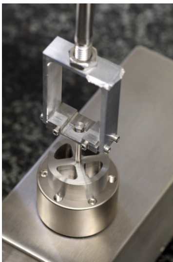
Fig. 3: Specially designed mass piece in carrier
