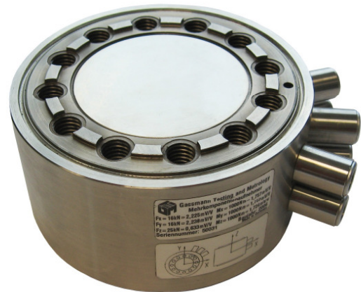
Fig. 1. Multicomponent Transducer of Monolithic Type
