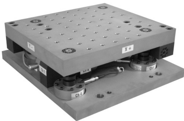
Fig. 3. Expanded Multicomponent Transducer of Platform Type
