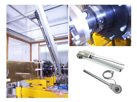
Figure 01 – System for calibration of Reference Torque Wrenches in the TSM (detail of the centralization parts and example of instruments).
