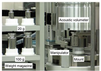
Figure 3 Photograph of the automated system
