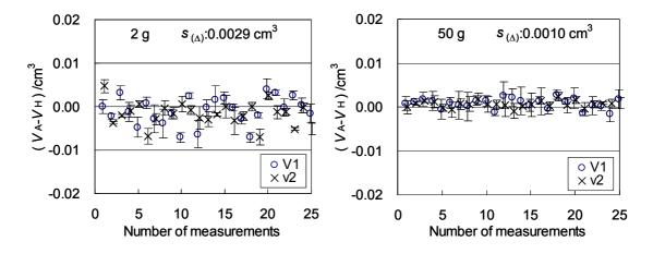
Figure 4. Deviations of measured values  $V_A$  from the reference volume  $V_H$
