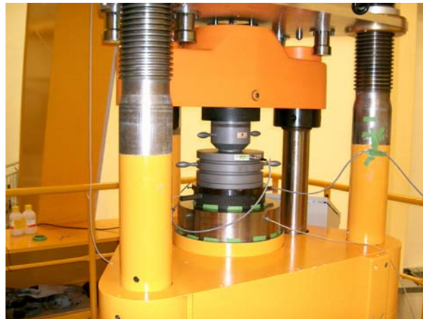
Figure 3 : Experimental scene in PTB 2 MN deadweight force standard machine
