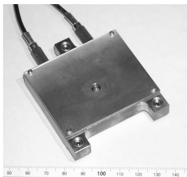
Figure 1. Capacitance cell showing the external leads to the upper and lower electrodes. The mass platen is visible through a hole in the top surface.
