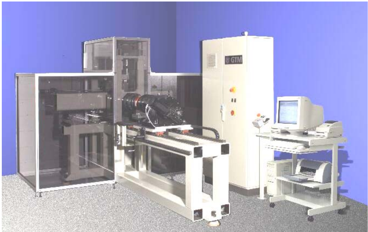
Figure 3: View of a 3 kN·m jockey weight machine (torque) at Dr. Staiger-Mohilo, Germany
