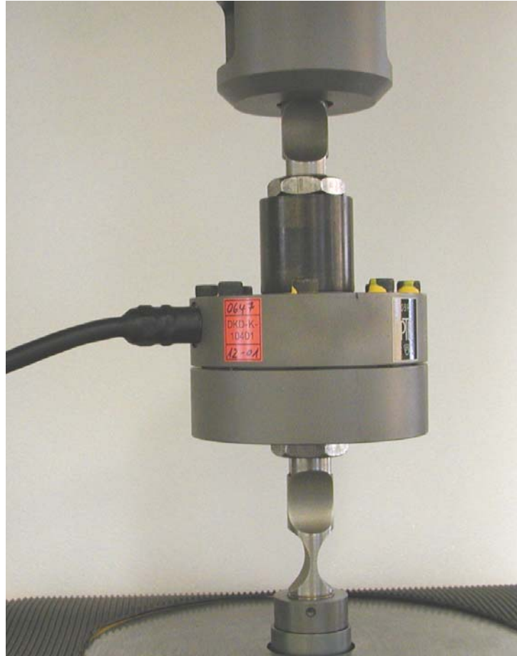
Figure 8: Test setup for loading with alternating forces
