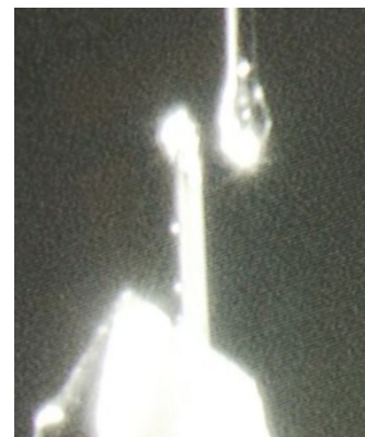
Fig. 3 The fiber probe (top) and the micro force sensor (bottom)
