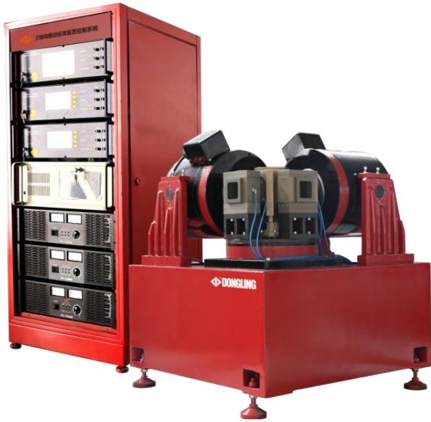
Fig.1 The air bearing three-component shaker
