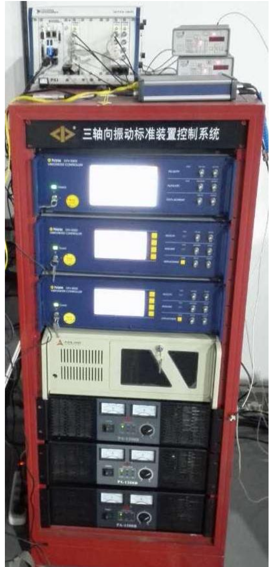
Fig.3 The sinusoidal three-component control system
