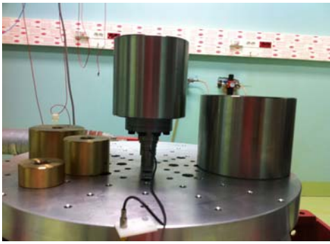
Fig 2: View of the masses and the adaptor used for that purpose also connected to a sensor.
