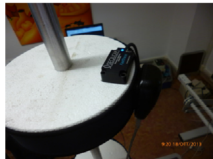
Figure 18. Tri-axial MEMS reference accelerometer and the postural reader fixed on the support at the vertical bar.
